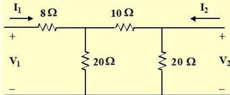
14(a) Apply Thevenin's theorem , find the equivalent circuit across the terminals A-B for the circuit shown below.
